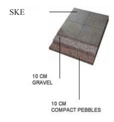
Tiles should be placed with a 3-5 mm joint onto a substrate made up of a first layer of gravel and pebbles (15-20 cm) and a second layer of sand (5-10 cm). This allows for the dry-installation with no need for adhesives and grouts. With some simple measures the laying of SKE tiles can be performed in complete safety without requiring specific equipment or the intervention of specialized personnel.
